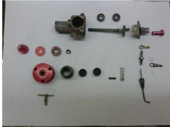
Fig. 3. Despiece Motor MK 17
