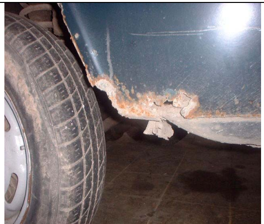
Fig. 20. Retention of deposits and water. Observe the deterioration that originates the accumulation of deposits and water due to poor drainage and anticorrosive treatment.
