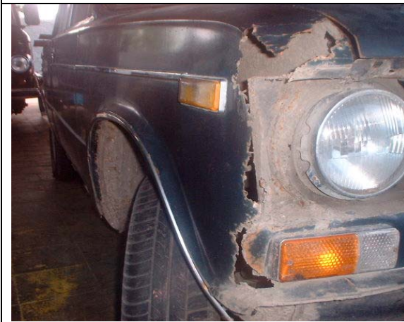
Fig. 19. Retention of deposits and water. Observe the deterioration that originates the accumulation of deposits and water due to poor design and anticorrosive treatment.
